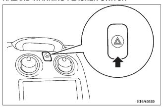
Press the flasher switch and the front and rear turn signals will flash intermittently, as the hazard warning lights. This is an emergency warning system and is not intended for use when the vehicle is in motion.
